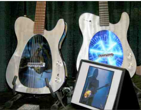
The Video Guitar, by Visionary Instruments. This actually has a video screen built into the body of the guitar. It can be hooked up to a computer to control the video being displayed
