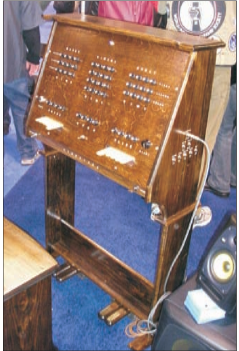
The Hymnotron, as seen at the Dewanotron Booth. The Hymnotron is a just intonation tone organ that uses a binary key arrangement
