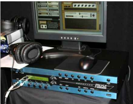
The Muse Receptor can process bass, guitar, and electronic drums at the same time.
